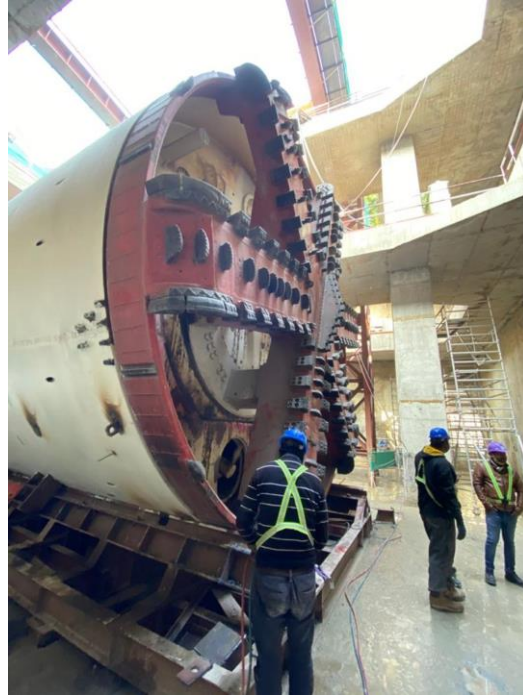
DMRC DC-06 Tunnel Boring Machine 5.8 m dia
