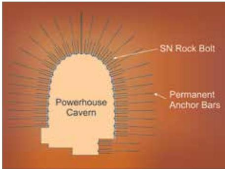
Permanent anchor bars used to support structure 7900 cubic meters. Due to poor geology, the shotcrete grade was changed from M25 to M35 in powerhouse construction.
