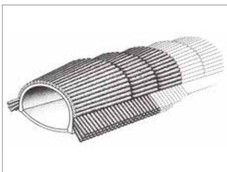
Pipe roofing used for excavation of headrace tunnel
