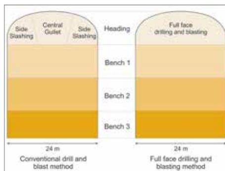
Full face drilling and blasting vs conventional method
