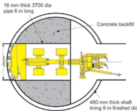
The TBM kept boring till around 200 meters towards the Ruparel shaft. Subsequently, the gripper was removed from the Mahim shaft to make room for muck removal, dewatering and other ancillary activities. This operation not only saved the cost of digging the tail tunnel and assembly tunnel and later refilling it, but also saved a lot of time as the maintenance and assembly of the TBM could be executed in the already excavated space.
